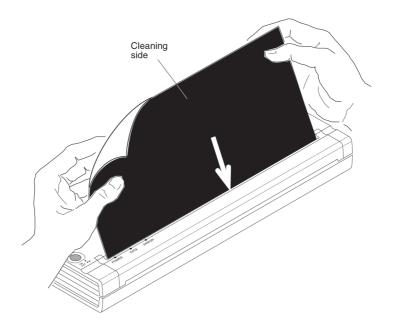
Figure 18. Cleaning the platen roller.
